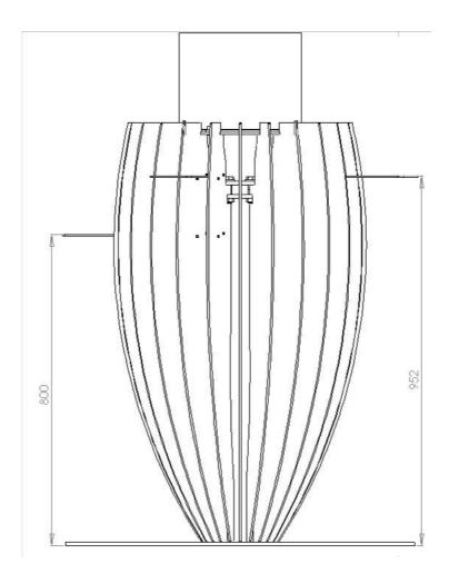
Placement of the 4 supports in the position chosen (height 800 mm/953mm).
